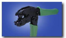
Designed for fully shielded plug, TDS8PC5, to crimp both contacts and strain relief at the same time.
